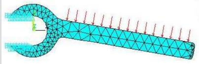
Boundary conditions ux = uy = 0 were applied along the lines where the wrench contacts the bolt. The mesh was refined to eliminate element-solution stress contour discontinuities. The following plots of von Mises stress show a maximum value of 39,333 psi at the fillet radius on the underside of the wrench.
