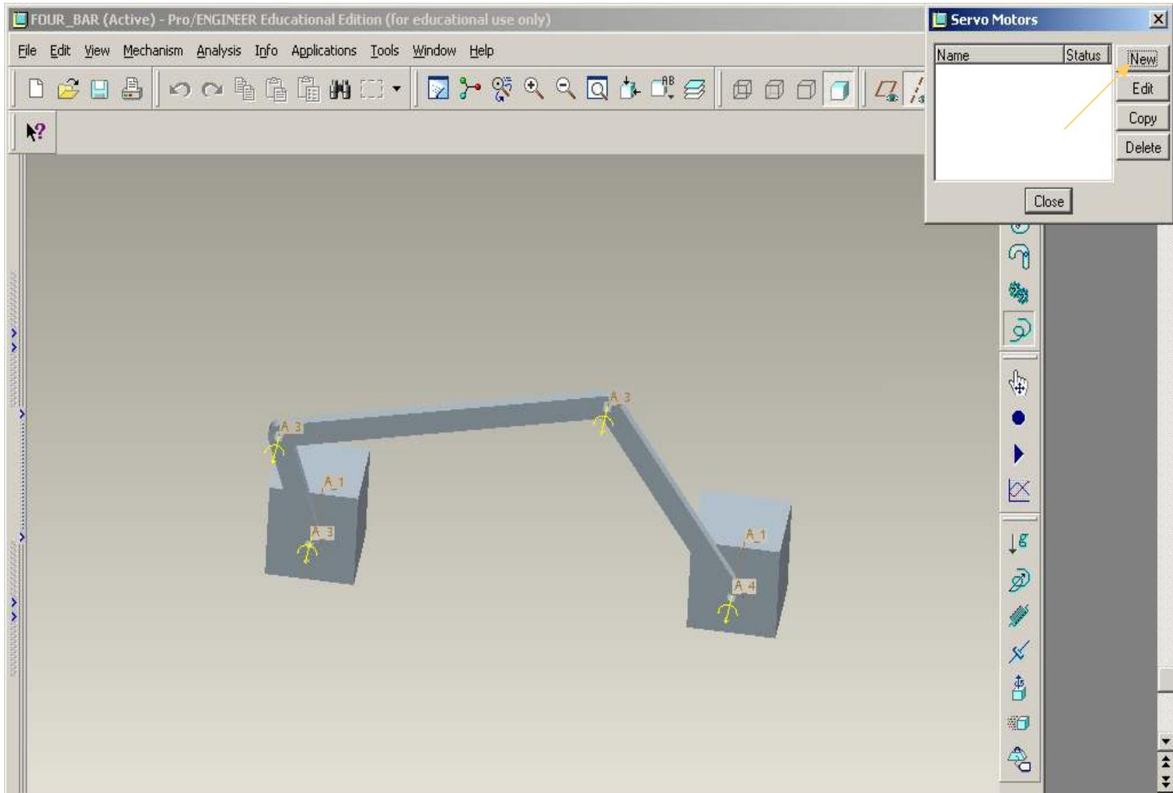
Click on **New** button to define the parameters of the servo motor.
