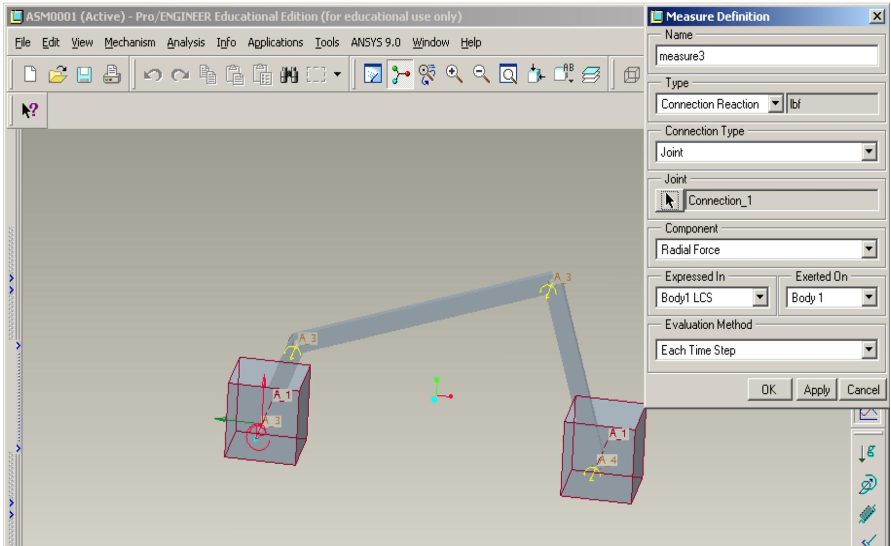
Select **JOINT 1** > component to be plotted – Radial Force > OK
