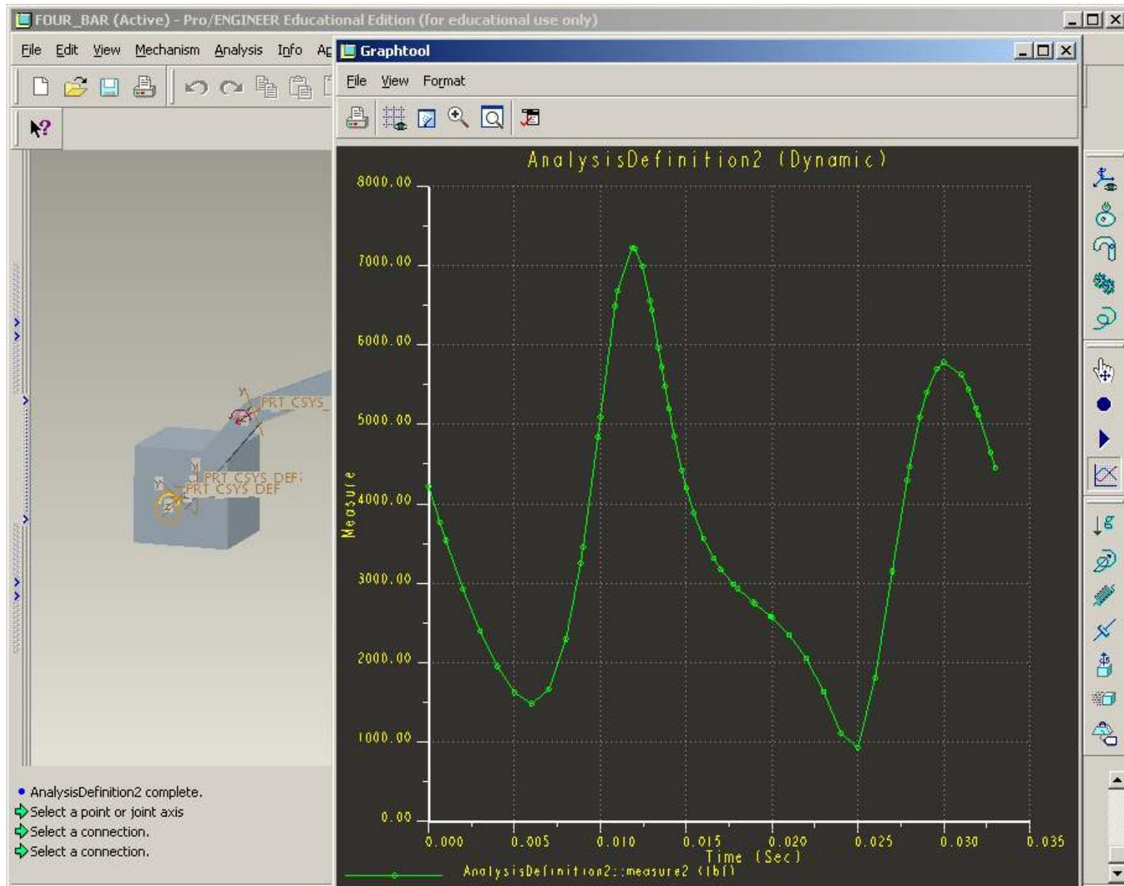
The Graph shows the Connection Reactions at **JOINT 2**.
