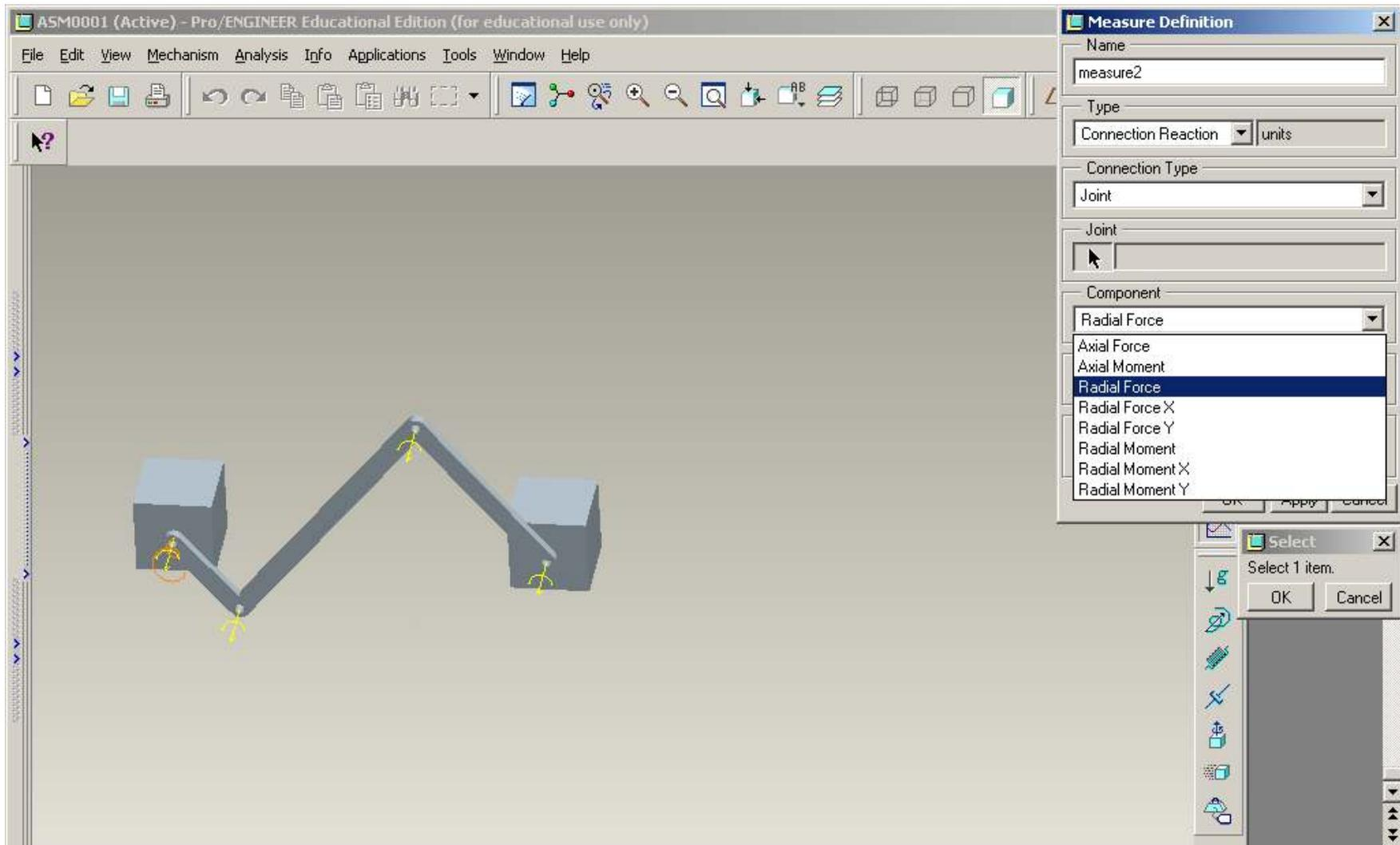
Select the joint and the measure to be plotted onto the Graph.
