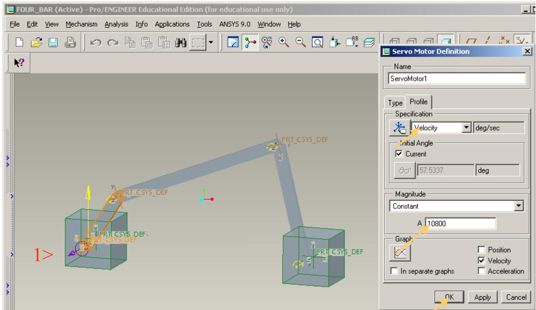
Select the **JOINT 1 axis** indicated by orange colored arrow to be the servo motor axis. > Enter 10800 > OK > Close
