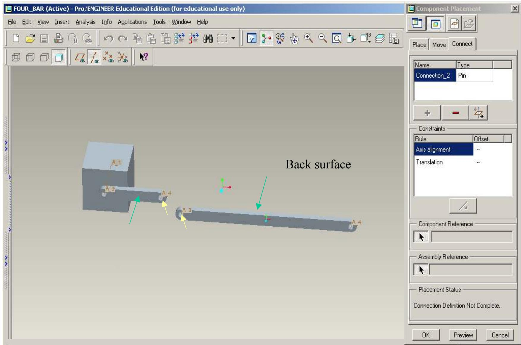
Keep the default “Pin” joint > Axis Alignment > Select A4 and A3 axes (Yellow Arrows)
