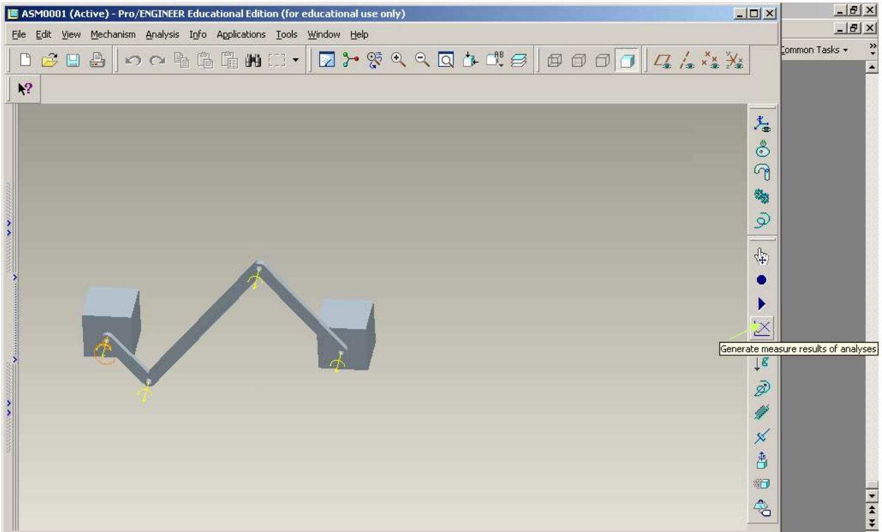
Select **Generate Measure Results of Analyses** to obtain the value of forces on the selected joints.
