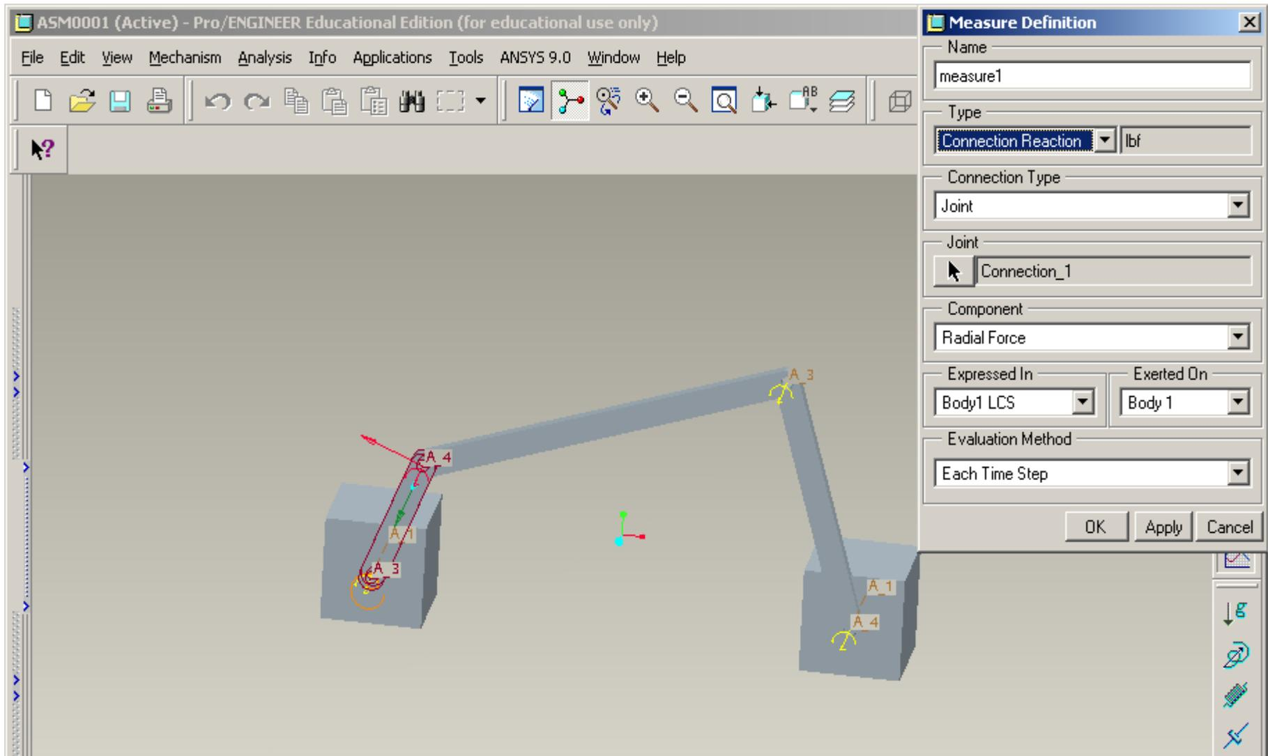
Now the **JOINT 2** is selected and component to be plotted – Radial Force > OK.
