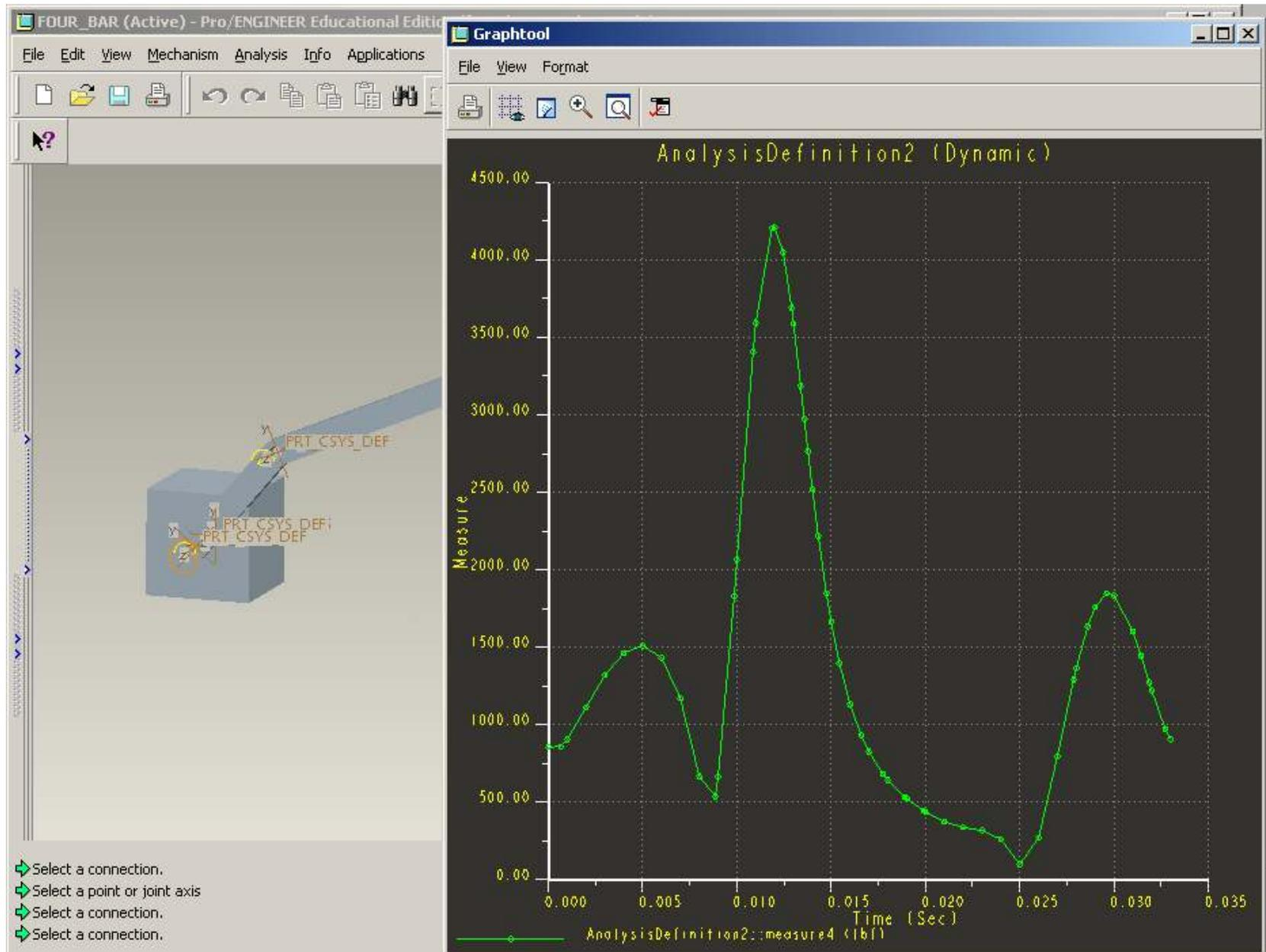
The Graph shows the Connection Reactions at **JOINT 3**.
