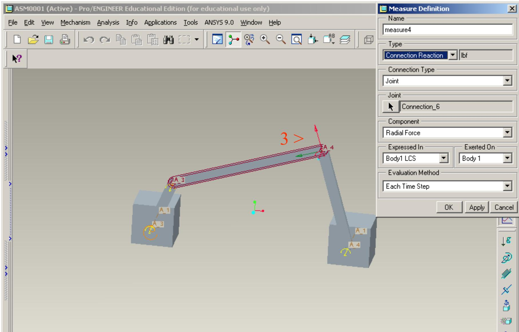
Select **JOINT 3** > component to be plotted – Radial Force > OK
