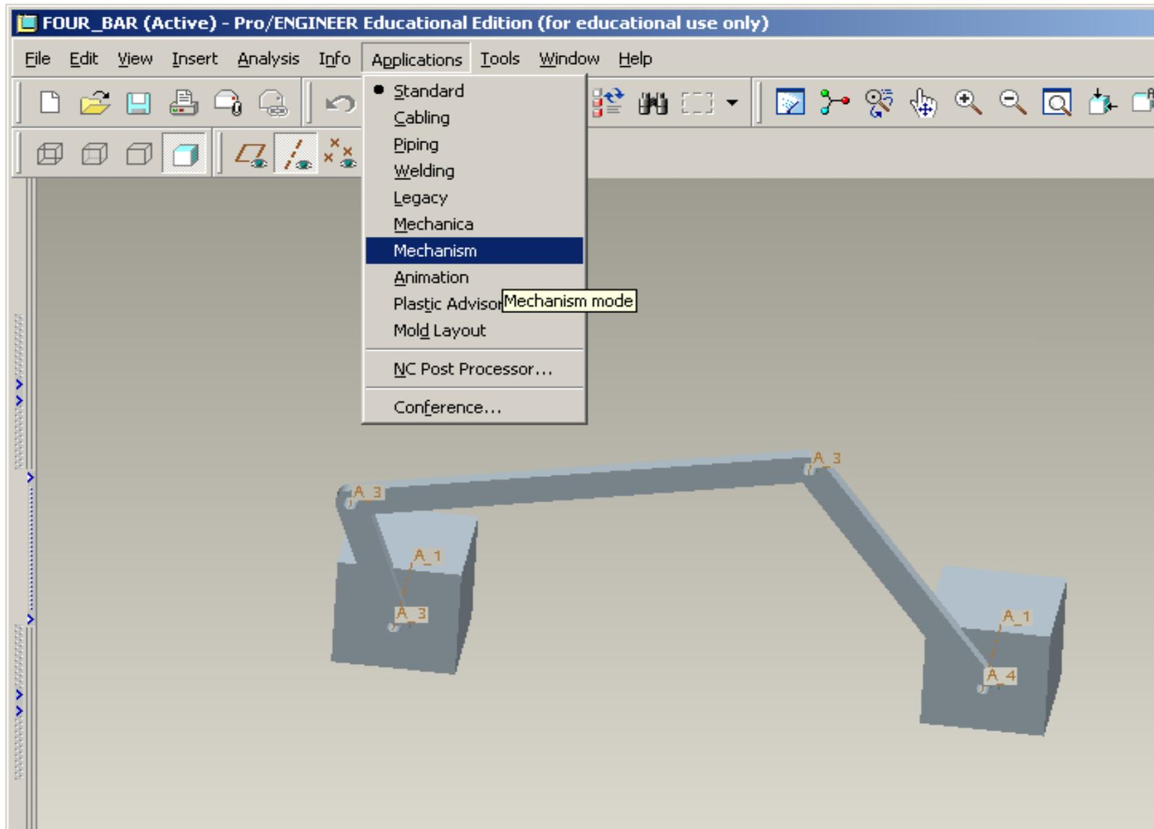
**Mechanism Mode** – Select Mechanism option from the menu bar.
