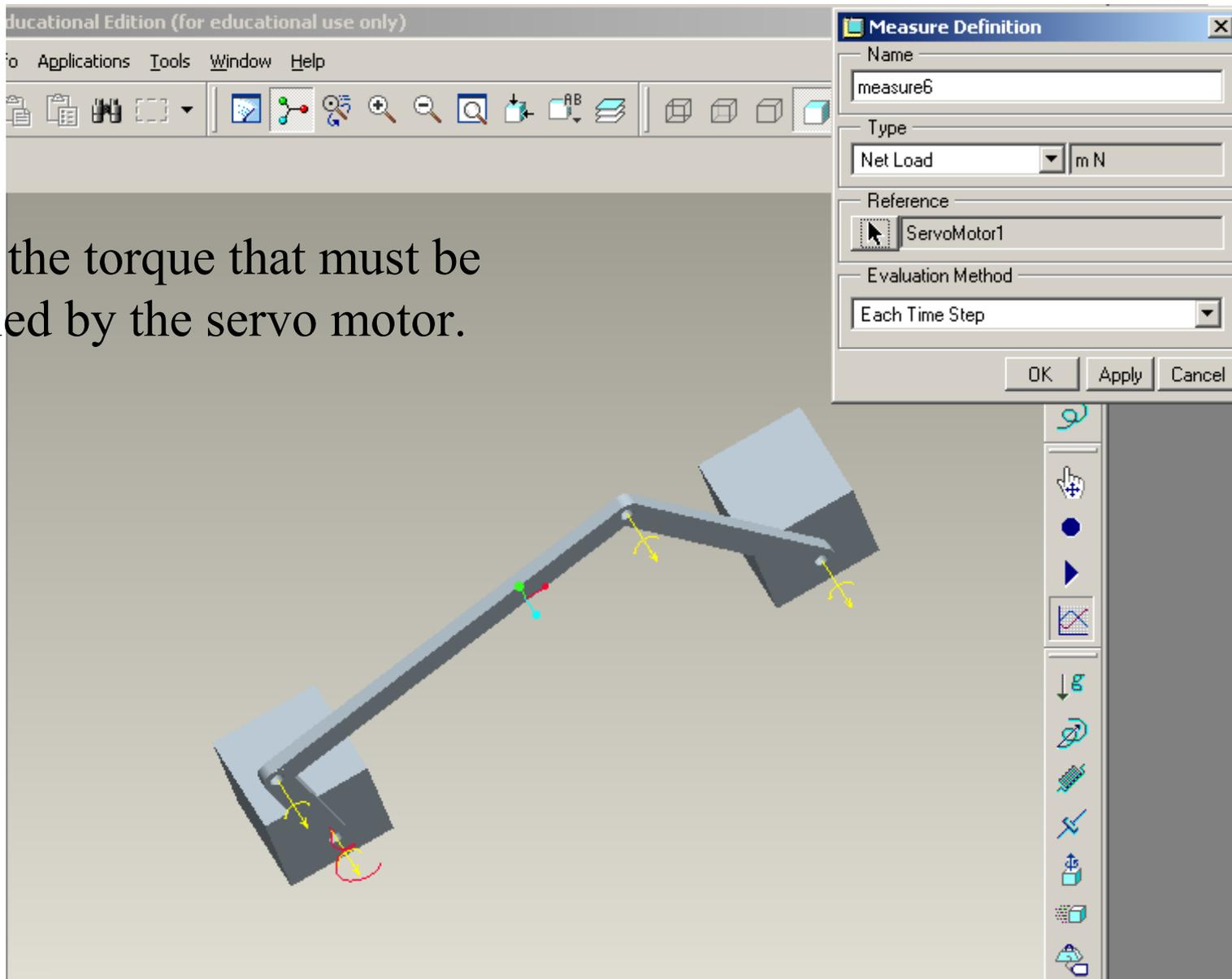
Create new measure > Net load > (pick the servo motor)
