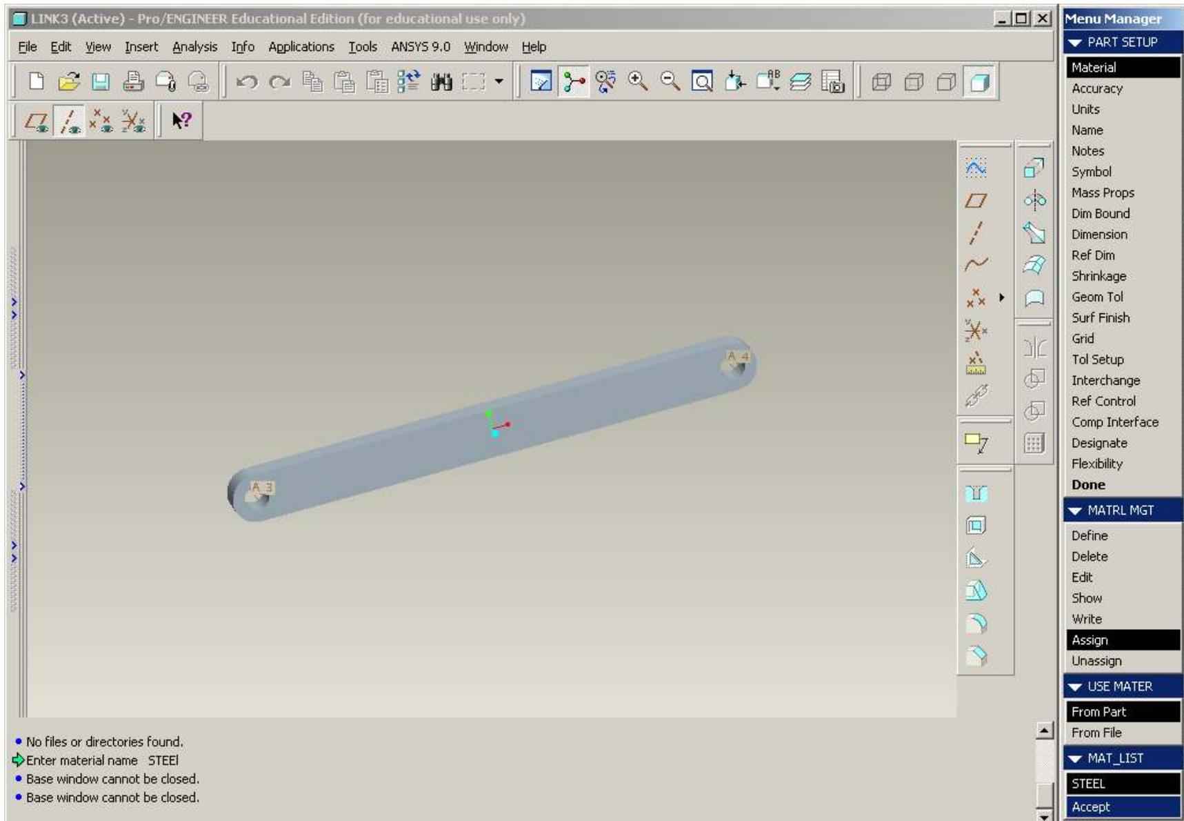
Edit > Setup > Material > Assign > From Part > STEEL > Done
