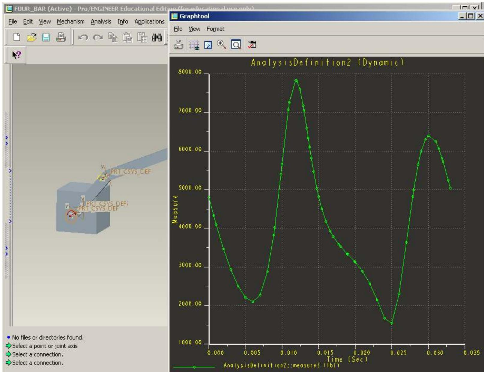
The Graph shows the Connection Reactions at **JOINT 1**.
