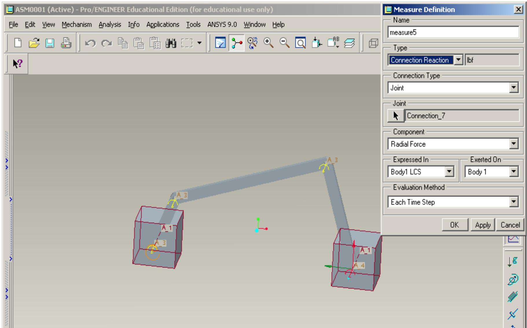
Select Fourth Joint > component to be plotted – Radial Force > Ok
