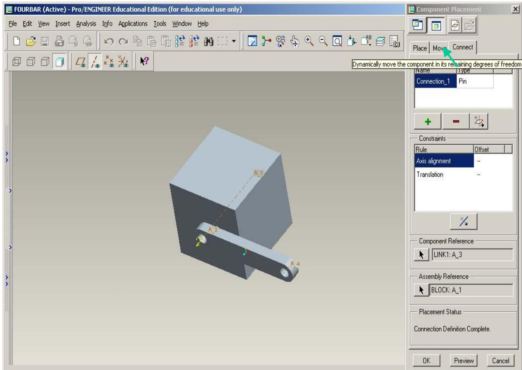
Click on Move Tab and rotate the link to required position
