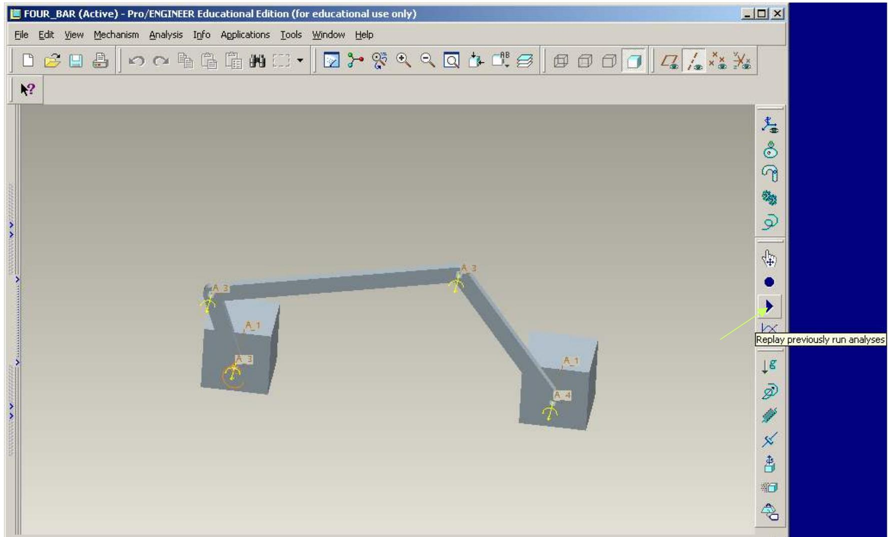
Select **Replay previously run analyses** to display the motion.
