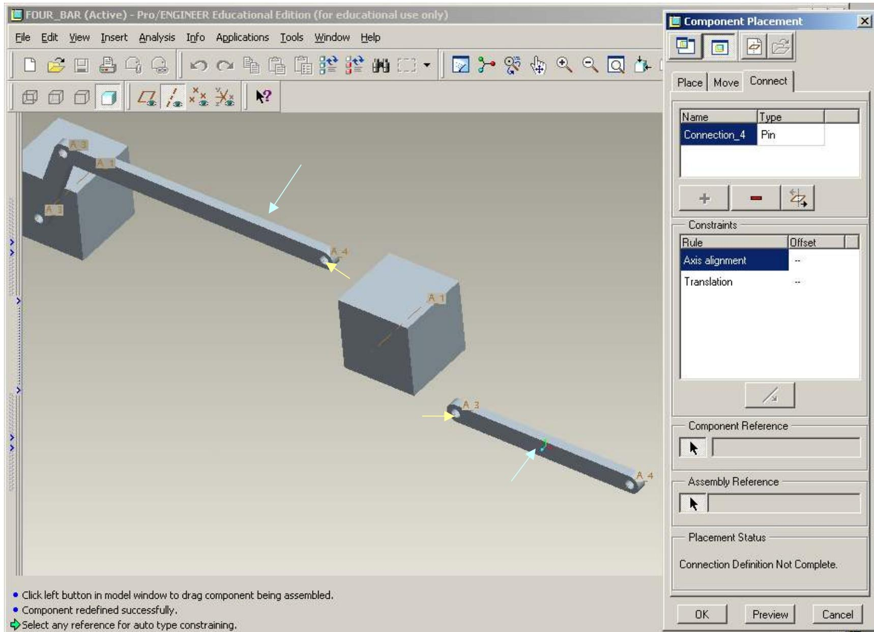
Keep the default “Pin” joint > Axis Alignment > Select A4 and A3 axes (Yellow Arrows)
