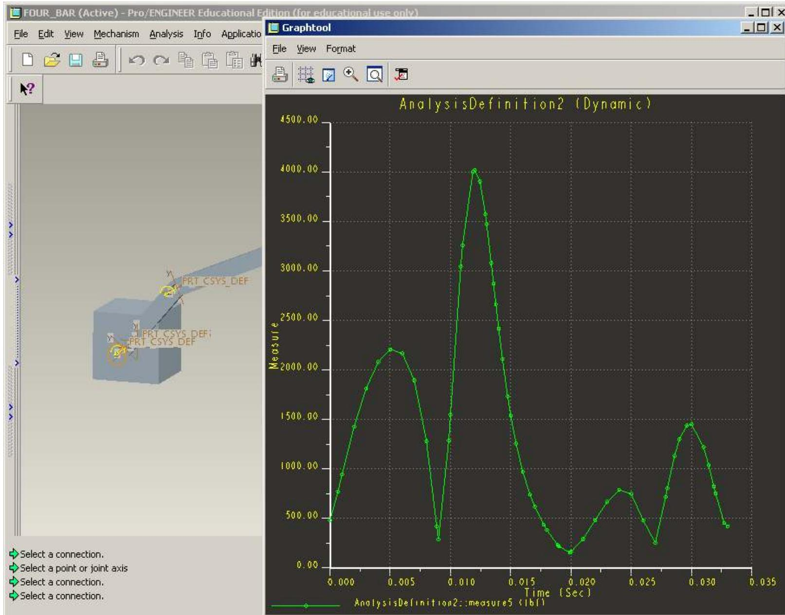
The Graph shows the Connection Reactions at **JOINT 4**.
