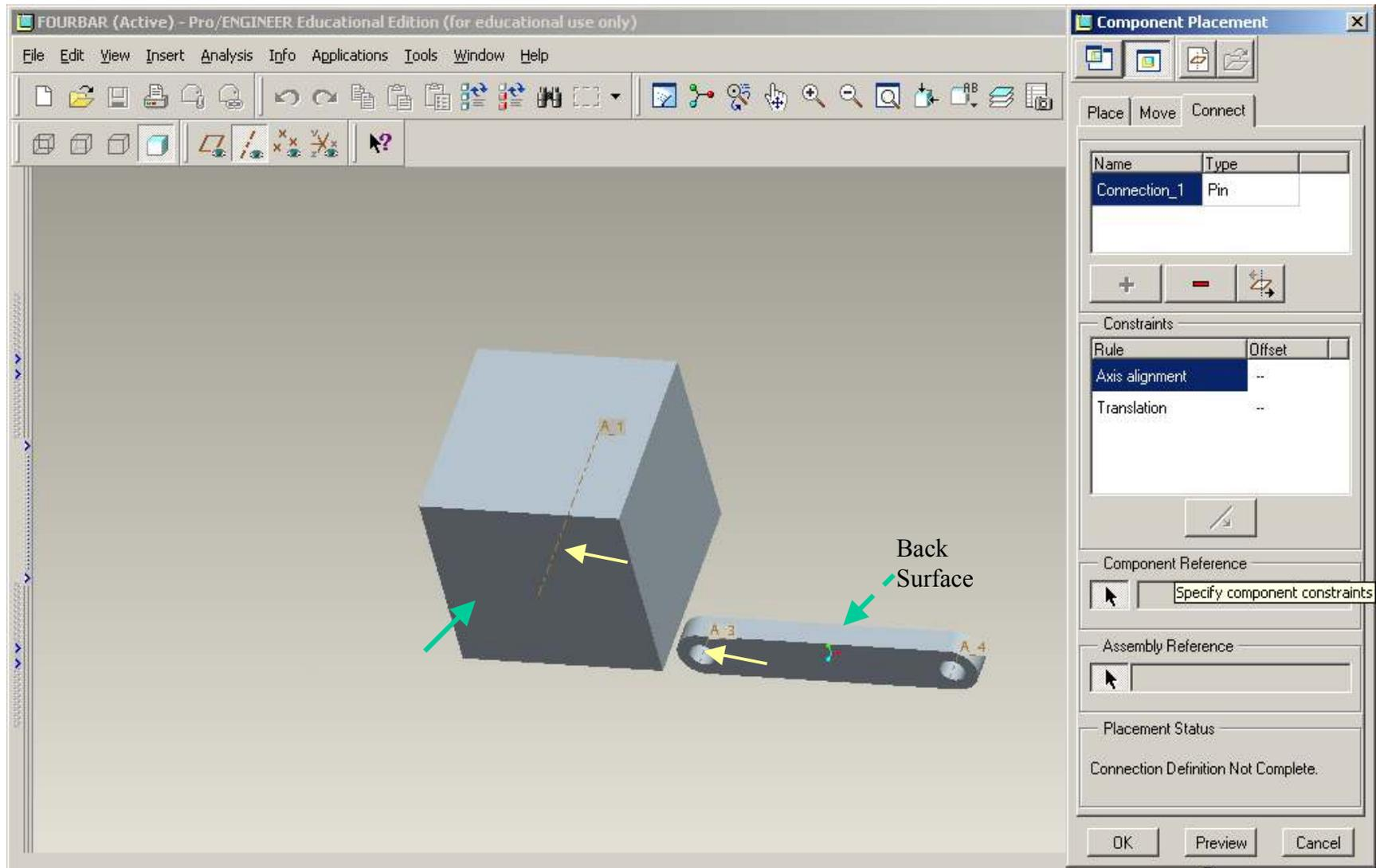
Keep the default “Pin” joint > Axis Alignment > Select A1 and A3 axes (Yellow Arrows)
