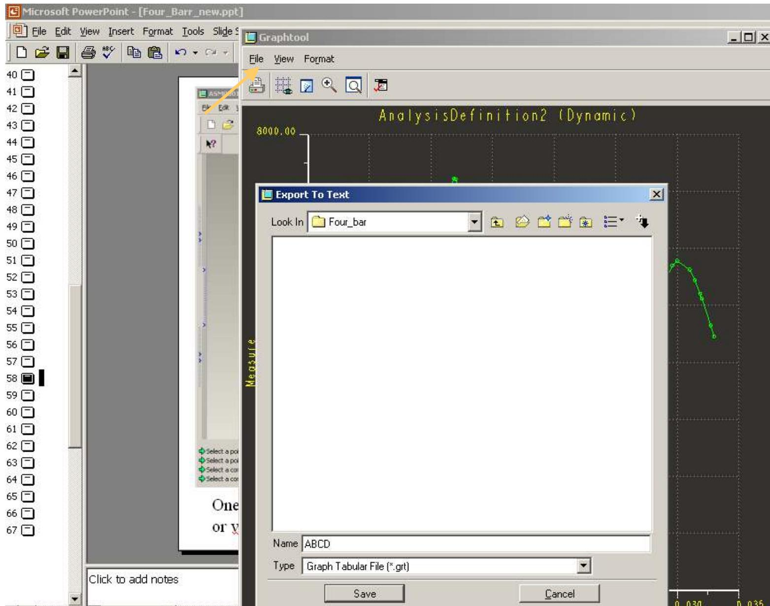
One can also write the results into Text file. Later this can be opened in notepad or wordpad.
