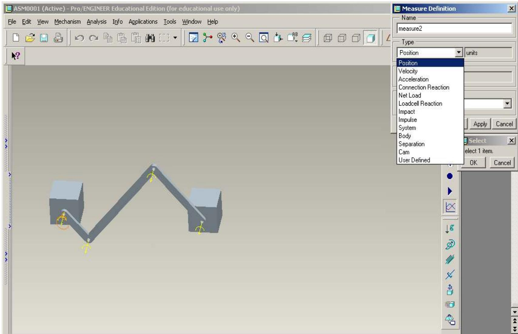
Select **Connection Reactions** to obtain Reactions at the joints.
