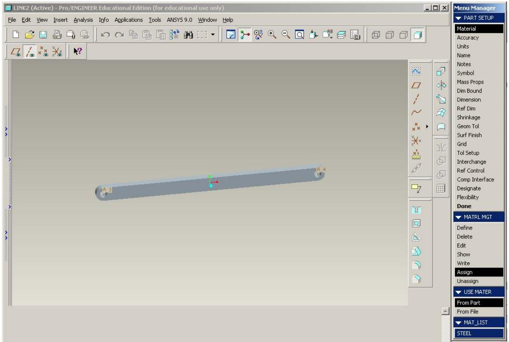
Edit > Setup > Material > Assign > From Part > STEEL > Done
